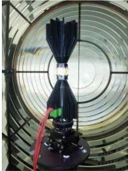
*A Research & Radio Navigation (R&RNAV) LED array light source inside a lighthouse optic.*
